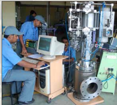
Dynamic testing of recirc valve for GE Thermodyn for Buzzard oil field in the North Sea.
