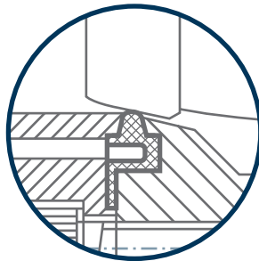
FIGURE 6. SERIES 65 – INTROL FIRESAFE DESIGN
