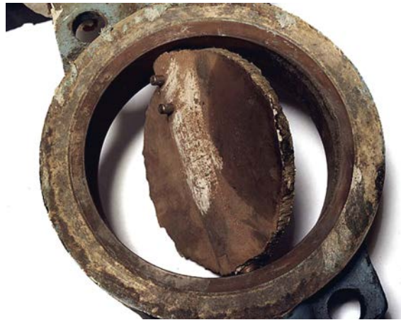
FIGURE 9. CAVITATION DAMAGE TO BUTTERFLY VALVE
