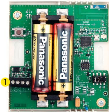
Rooms sensors can be mounted to the wall with screws or adhesive tape. Please note that the sensor is installed so that the black terminal strips are in the bottom left corner **1**.
