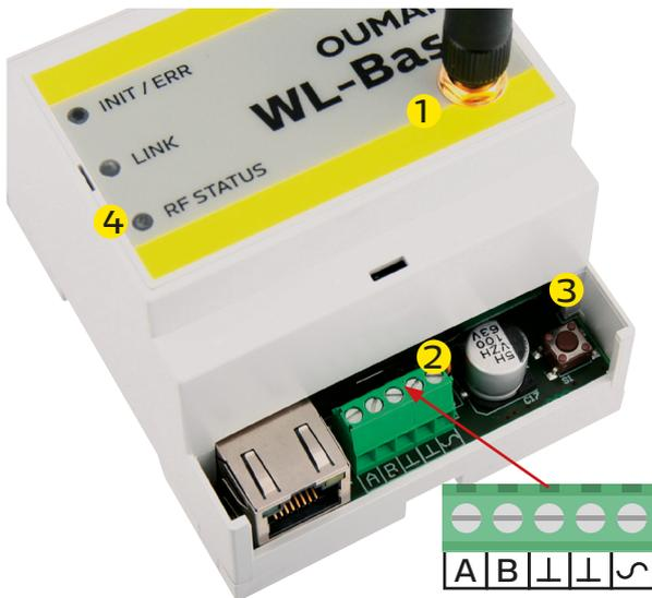
1. Connect the antenna (or the extra antenna with an extension cord) to the antenna connection of the base station. **Do not detach or attach the antenna when the base station is live!**
