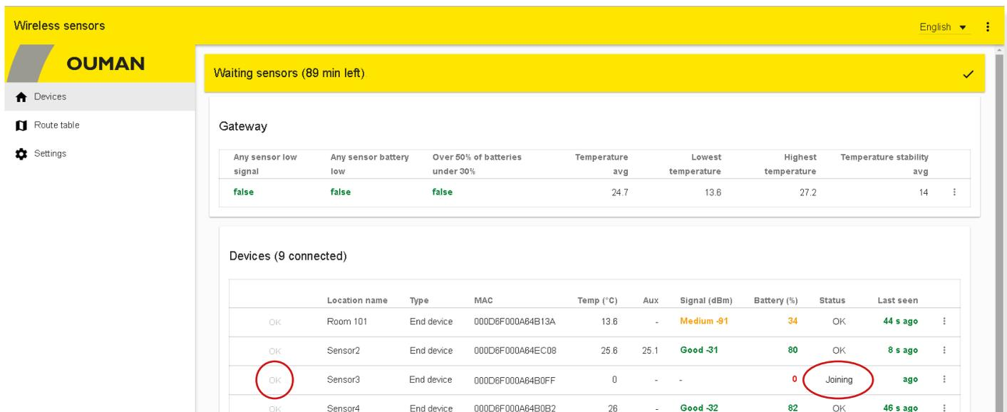
OK button – In the installation mode, the sensor sampling interval is 10 seconds by default. When there are 15 or more sensors in “join mode”, the sampling interval will slow down the device. When you press “OK”, the sensor’s sampling interval will change to two minutes, which will accelerate the device.
