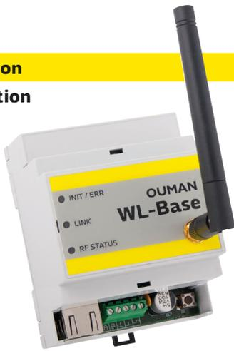
The base station is mounted to a wall or to the centre with a DIN bar. In the centre installation, the base station requires an external antenna. The base station must be installed indoors (0°C...+50°C).
